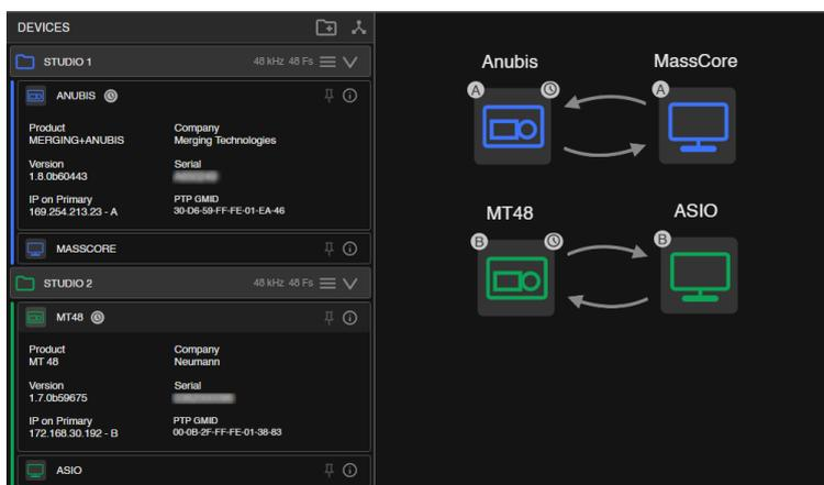
Each device shows a letter on its top left corner indicating a subnet. Devices of different subnets cannot generally be connected together.
